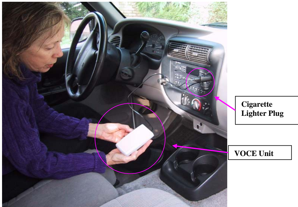
Figure VI.1 VOCE Unit for Collecting Vehicle Start Information
